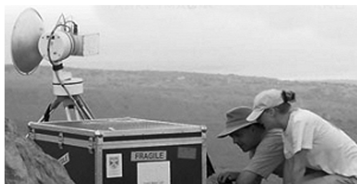
Figure 3 - Imaging the Montserrat volcano with AVTIS
