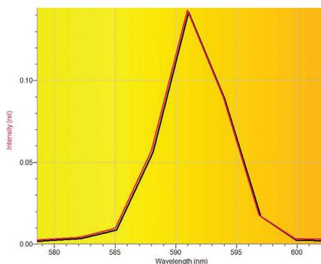
Figure 4 - Zooming in on the sodium yellow line (SpectroVis).
