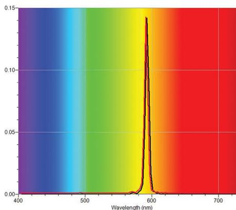
Figure 3 - Spectrum from sodium lamp (SpectroVis).
