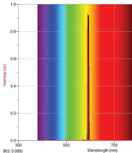
**Figure 11 - Sodium emission spectrum captured by Red Tide.**
