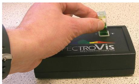
Figure 5 - Placing a cuvette in the cuvette holder.
