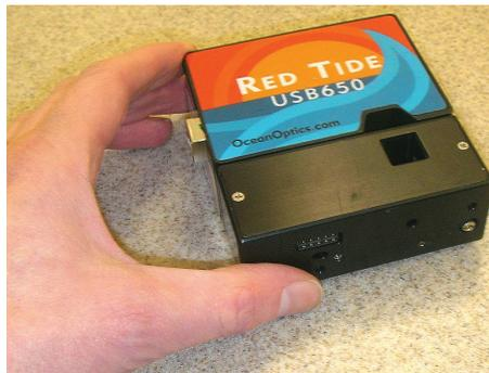
**Figure 10 - Red Tide spectrophotometer with optional cuvette holder (chemistry set).**
