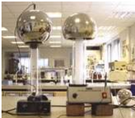
Figure 1 - Voltage measurement by means of standard air gaps. The dome on the right is being charged up. The dome on the left is connected to earth.
