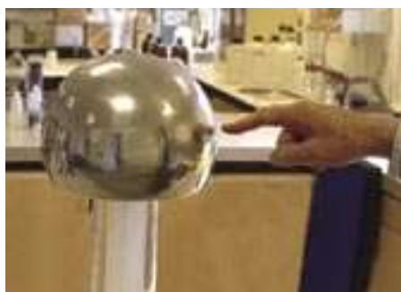
Figure 3 - Corona discharge through a projecting finger.
