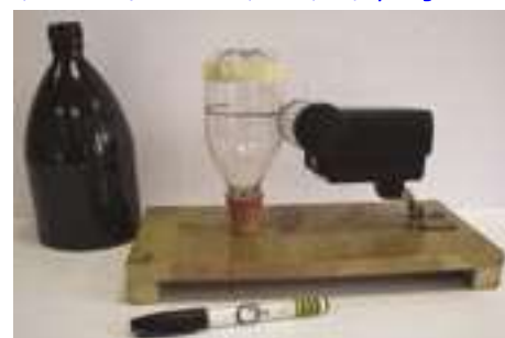
Figure 3 - Apparatus for larger-scale explosions of hydrogen & chlorine - only suitable for rooms with high ceilings or preferably in the open air.
