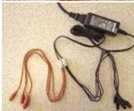
Figures 2a, b & c - Adaptations to connectors to allow up to 4 gel tanks to be connected to the one transformer.
