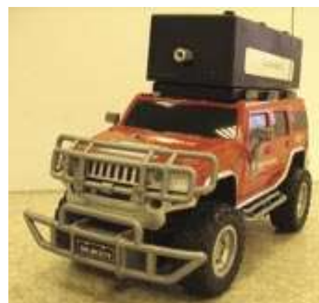
Figure 6 - WDSS mounted on radio-controlled car
