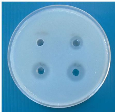
Figure 2 - The effect of different amylase solutions on casein breakdown. Clockwise from top: 2% NCBE bacterial alpha amylase (liquid), 2% bacterial alpha amylase (Philip Harris liquid), 2% bacterial alpha amylase (Philip Harris powder), 2% fungal alpha amylase (Philip Harris powder)
