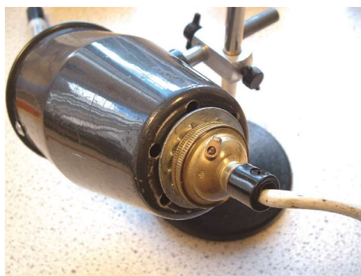
Figure 4 - Lampholder secured with shakeproof washer.
