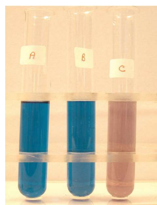
Figure 2 - B is tuned to change colour at 30°C
