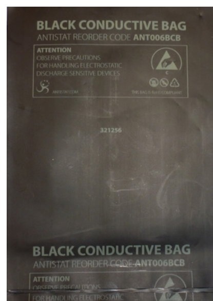
Figure 1 - Black conductive bag made from Velostat.
