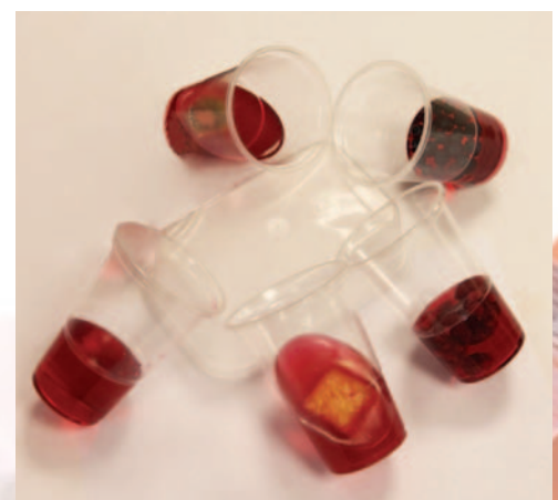
Figure 3 - Anti-clockwise from bottom left: Control - jelly with no added fruit (set), pineapple (not set) and raspberries (set), blueberries (set) and kiwi (not set).
