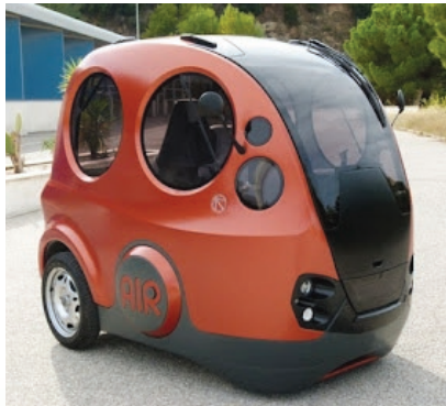
Figure 20 - This car runs on compressed air [4].
