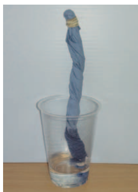
Figure 6 - The top of the stem is secured to a notice board with the double-sided tape while the base of the stem is submerged.
