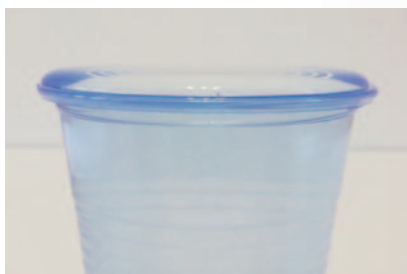
Figure 6 - Cup filled beyond the brim with water held in place by surface tension.
