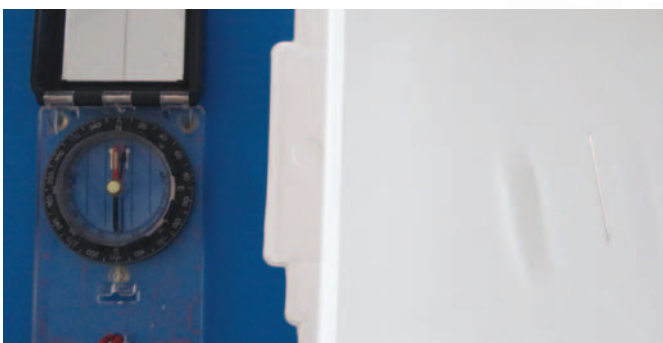
Figure 13 - Needle is held on the surface by surface tension and has aligned north-south.
