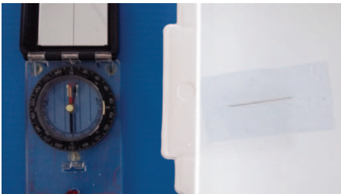
Figure 12 - Needle placed on tissue paper in an east-west alignment.
