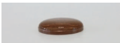
Figure 5 - Coin showing dome of water - maximum capacity before surface tension was broken.
