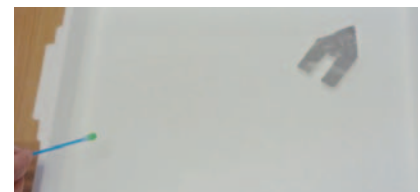
Figure 23 - After the washing up liquid is applied to the water surface near the stern, the boat moves across the tray.
