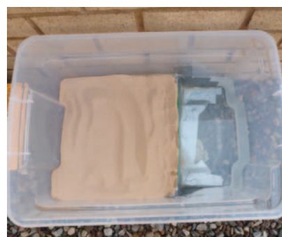
Figure 11 - Waterproof divider keeps sand in one section.
