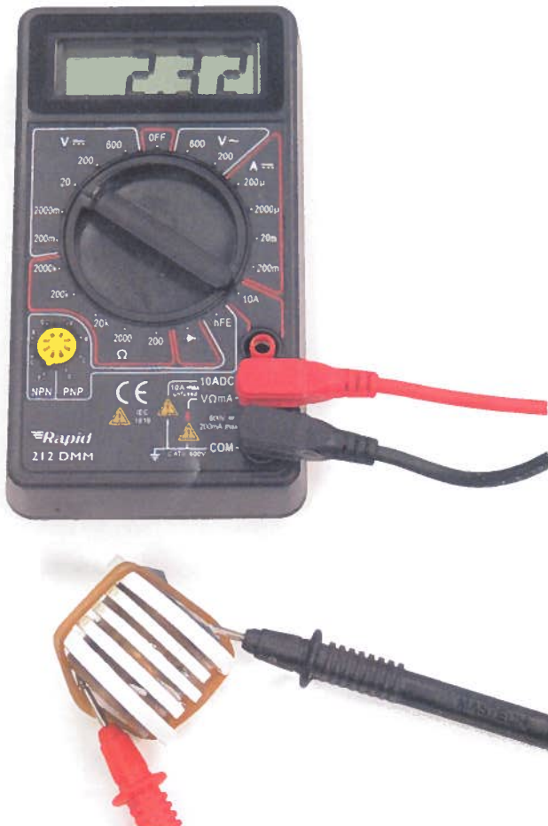
Figure 1 - Multimeter set to measure voltage and connected to the 'battery' of coins, foil and packaging discs.
