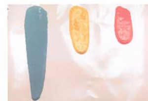
Figure 1 - A fair test set-up to compare putty runniness.
