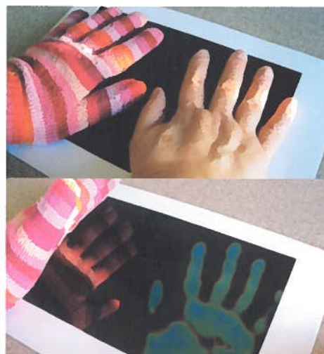
Figures 3a & b – Gloved and ungloved hand placed on film then removed.
