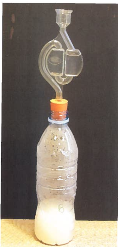
Figure 4 – Plastic fermentation lock (airlock) which can be obtained from local home brewing suppliers or on-line supplier [1].
