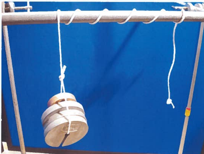
Figure 1 – Using friction to hold things up
