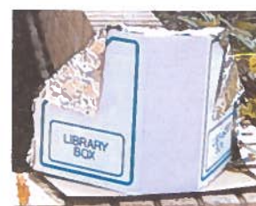
Figures 12 & 13 - DIY solar cooker (front and rear) made from aluminium foil and a cardboard library box.
