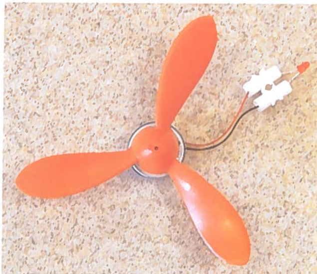
Figure 9 - Model turbine (propellor, terminal block & red LED)
