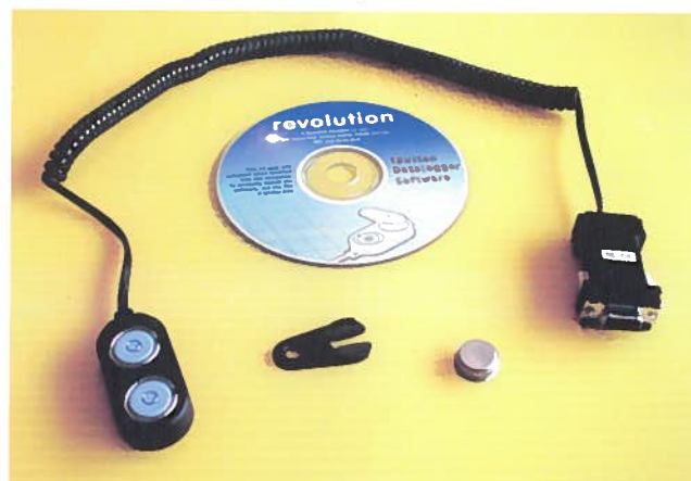
Figure 2 An iButton kit: iButton port and serial lead, iButton and CD ROM.
