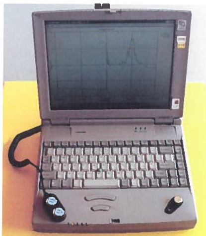
Figure 1 An iButton port connected to a laptop computer with an iButton , in its holder, on the reader's right.
