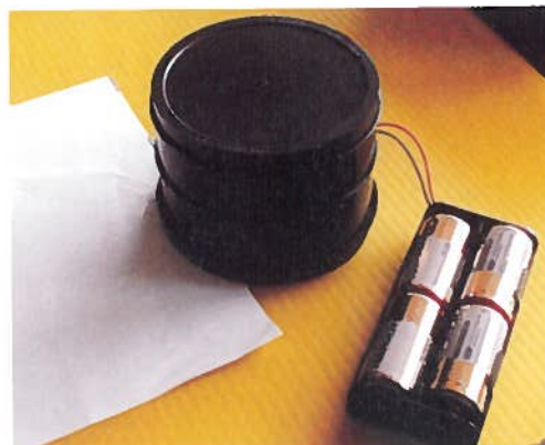
Figure 4 Economy light box (Ossie) in use with batteries. No dim-out.
