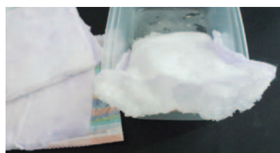
Figure 3 - The saturated nappy. The hydrogel can hold no more water.
