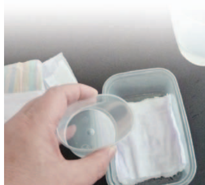
Figure 2 - Pour small measured quantities of water onto the nappy.
