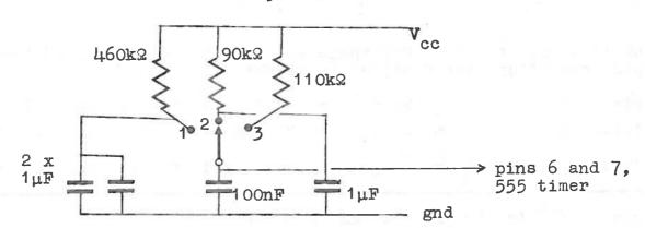
Fig. 5. Frequency range switch. Position 1 = frequency in Hz; position 2, x10; position 3, x100. Resistance values are approximate, and must be adjusted to give 1 s, 100 ms, and 10 ms pulse lengths.
