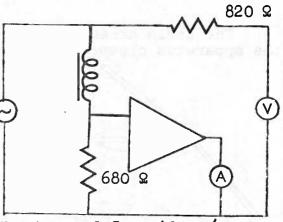
Circuits for H320/3 and H3020/3. Chart speed 5 or 10 mm/s. V and i are recorded on different channels of the recorder.
