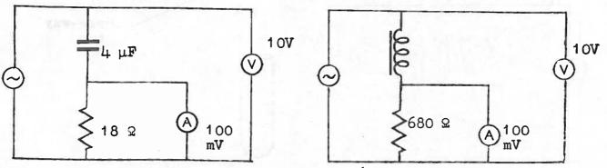
Circuits for CR503. Chart speed 10 mm/s. 10 V and 100 mV are the respective sensitivity ranges for V and i.
