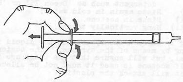
If the finger and thumb are squeezed inwards, in the direction indicated by the curved arrows, the plunger is pulled gently outwards and is under complete control. For movement in the opposite direction the plunger is pushed in, using the finger and thumb as stops against the top of the barrel. In both cases, extended movement in one direction will require adjustment of the position of the finger and thumb on the plunger from time to time.
