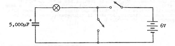
The switches are either biased toggles or Push-to-Test switches. Both types are spring loaded so that they return to the OFF position when released, and are available from Radiospares.
