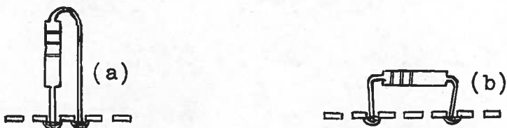
Fig. 5. Two methods of mounting components on Veroboard.
