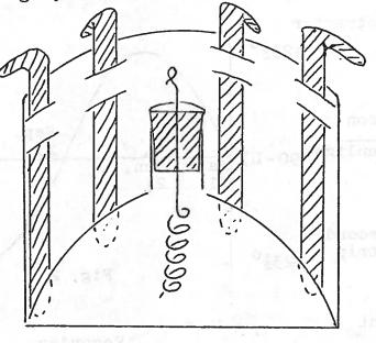
The apparatus to be described illustrates that there is no tension in an elastic band supporting an object when both are falling freely. The object is a hardboard plate, which is arranged to be in free movement between vertical guides in a hardboard support, to which the "fixed" end of the elastic band is attached. The remainder of the apparatus consists of a mechanism to ensure quick and clean release of/ of the falling part, also made from hardboard.
