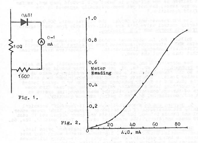
Two refinements which we found convenient and which add little to the cost of the equipment are (i) to substitute for the  $10\Omega$  fixed resistor a  $25\Omega$  variable rheostat, also from Radiospares. This can then be used to adjust the initial meter reading to a suitable value nearly or at full scale deflection. The second was to connect a  $1,000\mu F$  6V electrolytic capacitor across the meter. This removes the tendency on the part of the pointer to vibrate at 50~Hz.
