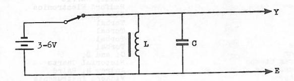
L is the 250 turn section of Unilab LB-3 coil, with a single C core inserted; C is a 4µF paper capacitor and the switch is made up by inserting a piece of copper foil in place of the normal tape in a ticker timer. This gives a recurrent switching action at 50 Hz,/
