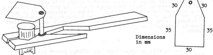
The small flap of hardboard is hinged on a round peg of wood which can be push fitted into the central hole of the spring of the testtube holder. Thus it can be swung to one side for pouring operations.
