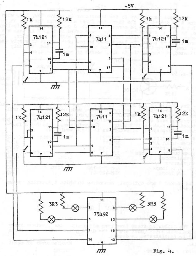
As in the previous case, the indication is given on a 4.5V, 0.3A low voltage lamp bulb. If something more powerful by way of an indicator is wanted then thyristors or triacs are the answer. Because we do not like direct connection between t.t.l. circuits and mains voltage, and because we have a large number of 100V thyristors going cheap, we experimented with circuits which would drive a raybox lamp. The circuit shown (in Fig. 5) has been tested and found to work.
