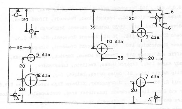
Drilling of aluminium panel, viewed from underside. All dimensions Holes marked A are No. 33 B.A. twist drill. in mm.
