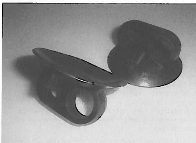
Figure 6 Set of rubber suction pads which may be used as Magdeburg hemispheres.
