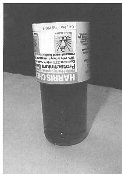
Figure 1 Philip Harris Protactinium Generator with cap upright in normal storage position.
