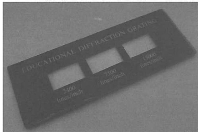
Figure 1 The original version of the Educational Diffraction Grating showing its imperial markings.
