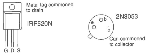
Figure 2 Pinouts for the MOSFET and bipolar transistors.
