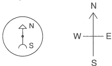
7 On removing the compass from the Major magnet's field you should find that it points north
