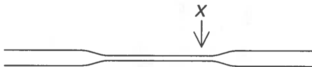
Figure 1. When glass softens, pull gently to form uniform narrow rod.
