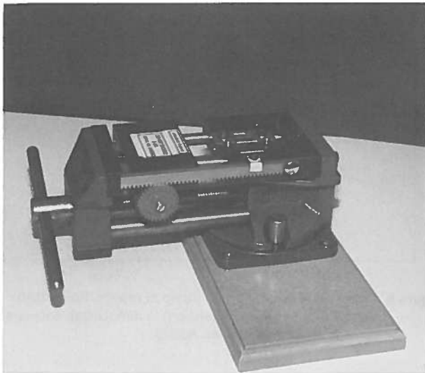
Figure 4 Test rig : modified vice with rack and load cell.
