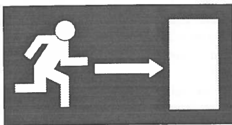
Fig.2 Another example is that Fire Exit signs cannot rely solely on the words in white on a green rectangle. There must be a symbol of a running man and, or, an arrow but the text can be appended alongside.
