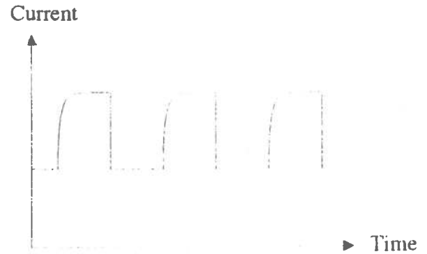
Figure 4 - Stepper motor - running slowly
