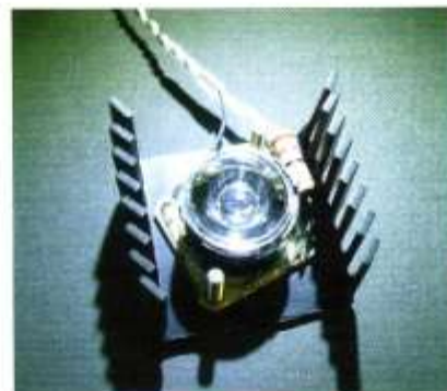
Figure 6 Lumiled (type: Luxeon 1W Star with Optic (Low Dome Batwing)) fastened to heatsink and with series resistors. Anode marked with copper dot (not shown).
