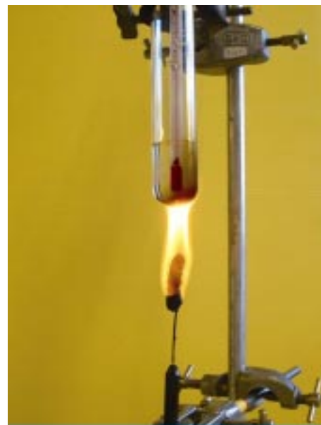
Figure 1 'Traditional' simple calorimetry. A piece of the proprietary snack - a 'Wotsit' burning on a mounted needle.
