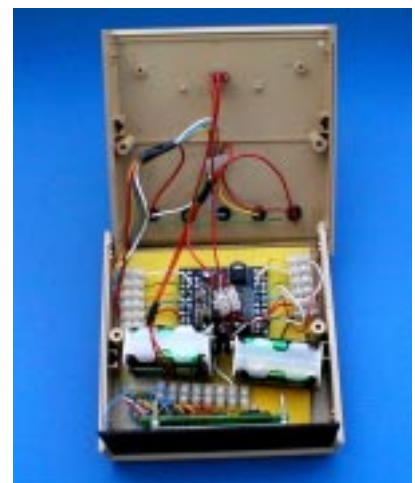
Figure 5 PICAXE board inside box.
