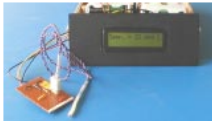
Figure 2 Picture LCD showing temperature with thermistor.
