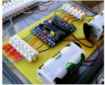
*Figure 6* Close-up view of PIC microconroller on top panel of toy washine machine.
