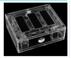
Figure 1 The Perspex case of the Solar Science Set with its 3 solar panels on the lid and showing 4 output devices down the left hand side.
