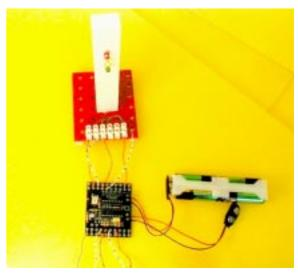
Figure 2 Fitment of bulbs and holders in model traffic lights.
