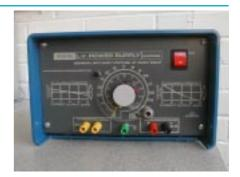
**Comments:** Performance is fair. The mean ac voltage is generally too high whereas the mean dc value is too low. Both fall faster with load than on some other similar products. The rotary switch resembles the one on Irwin's EJ1001 – therefore having the same inherent weakness but satisfactory performance. The price is a little high.
