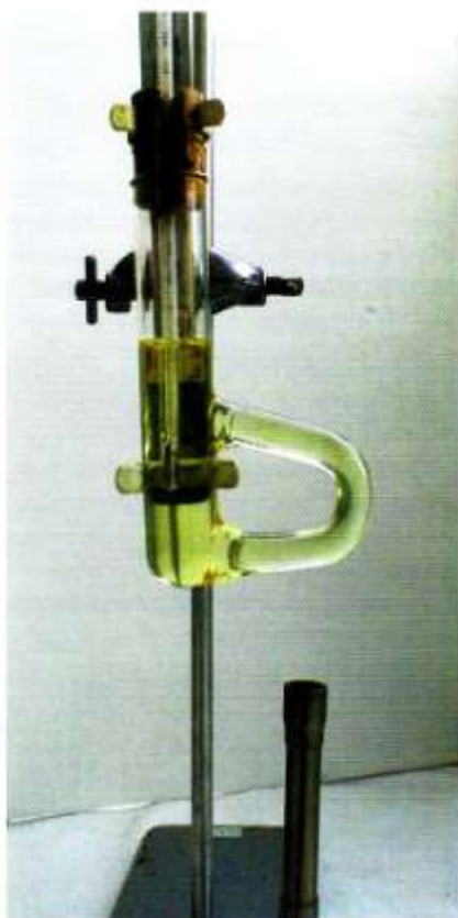
Figure 2 A Thiele tube set-up in use. (cf. Fig.3).
