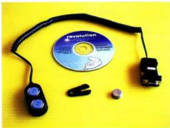
Figure 3 iButton probe, serial lead to PC, iButton Key (coin-size) and key fob (Clockwise from bottom left).
