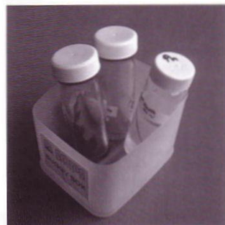
Figure 3 A SAPS 'Buggy Box' - a holder and carrier for Universal containers or McCartney bottles made from the base of a plastic (high density polyethylene or HDPE) milk container.
