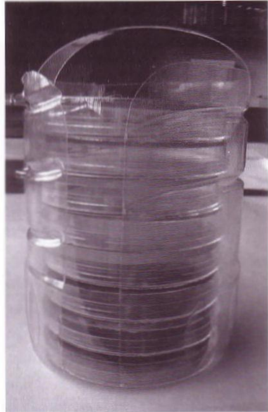
Figure 1 Photograph of a Petri dish carrier made from the base of a plastic juice bottle.
