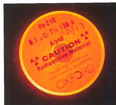
Figure 2 PASCO's alpha source with the radionuclide Po-210 – its disposal is very difficult. (Photo by CLEAPSS.)
