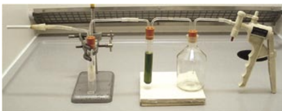
Figure 2 - Puffing model driven by a hand-operated vacuum pump
